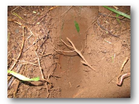
Plate 24. Though damp at the time of excavation, the soil pit at Sampling Point A3 revealed Paaloa silt clay that did not show hydric characteristics.
