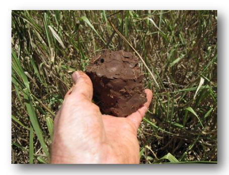
Plate 27. As expected, the soil surface at Sample Point A6 is deeply cracked. Samples are consistently hard, dry, dark reddish brown Helemano silty clay (2.5YR 3/4) with no evidence of hydric properties.
