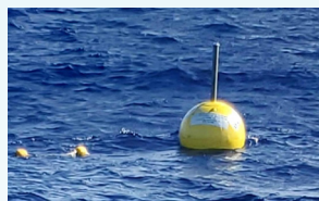
Echosounder attached to FAD #3 after deployment. Photo: Jaime Bass, DAWR.
