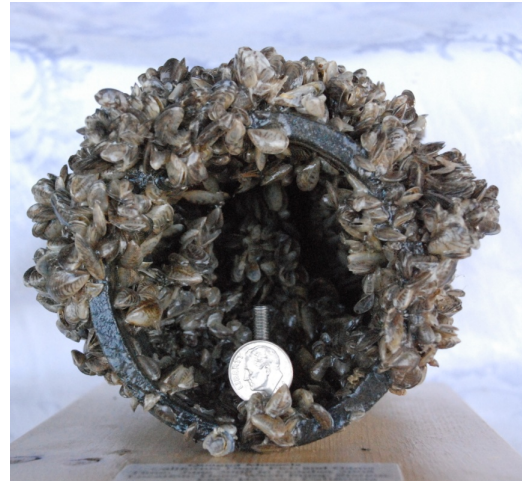
Figure 4. Photograph of quagga mussels clogging a pipe. Note the dime in the foreground of the photo for scale (dbw.ca.gov)
