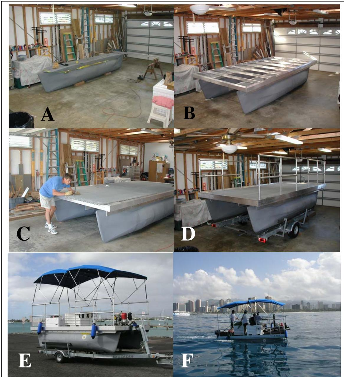
Figure 2. Various stages of barge construction for Supersucker Jr. A) Construction of 2 bow pontoons; B) Construction of framing for deck material; C) Installation of the deck material; D) Installed rails for barge deck; E) Completed barge at boat ramp; and F) Functional barge during first field test.
