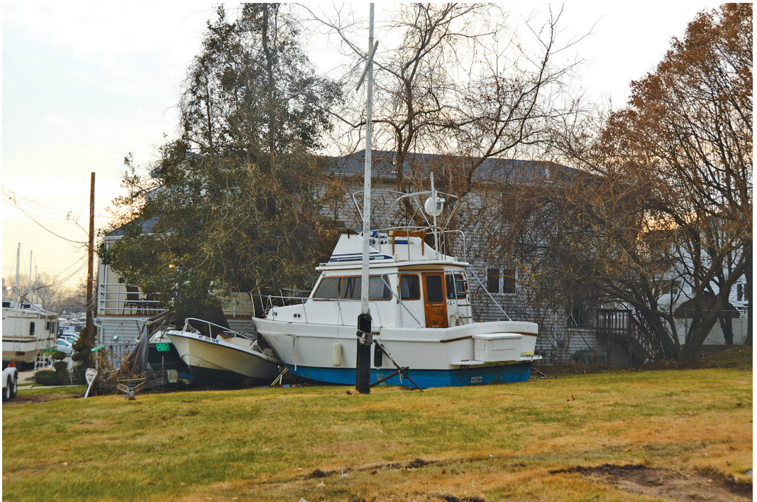
Storm surge from a hurricane is one of the greatest dangers to boats and marinas. It destroys structures and pushes boats inland. Hurricane Sandy in 2012 damaged or destroyed more than 65,000 boats on the east coast. Photo courtesy of Dennis Hwang.
