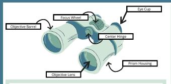
Binocular specifications contain two numbers, for example 8x42 - a great option for viewing forest birds. The first number is the magnification. The second number is the diameter of the objective lens.
