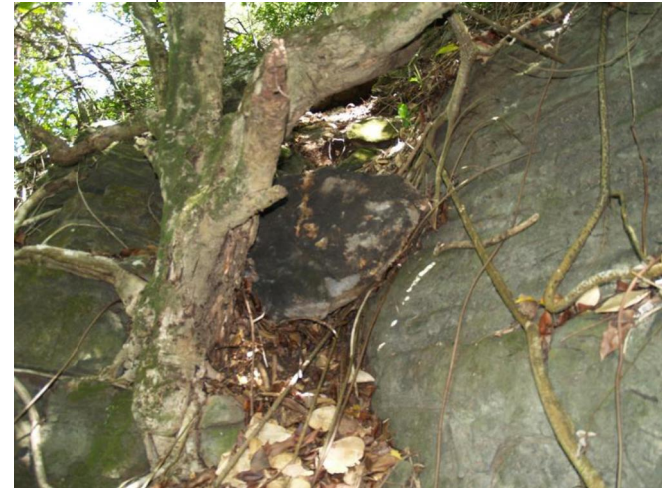
Photo 2-11. A recent rockfall boulder on steep slope with potential for further fall. Notice the fresh impact marks and tree barks on the boulder. At B18.
