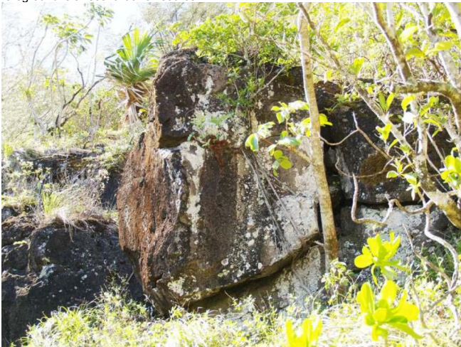
Photo 2-3. An overhanging and standing boulder with large opened back fracture At B4.
