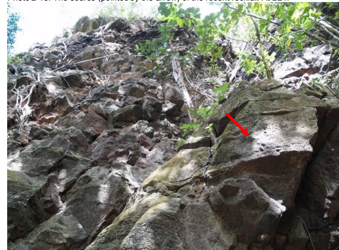
Photo 2-19. An overhanging fractured rock (pointed by the arrow) with potential for wedge failure. Notice fractured rocks on the cliff face at left of the photo. At B21.
