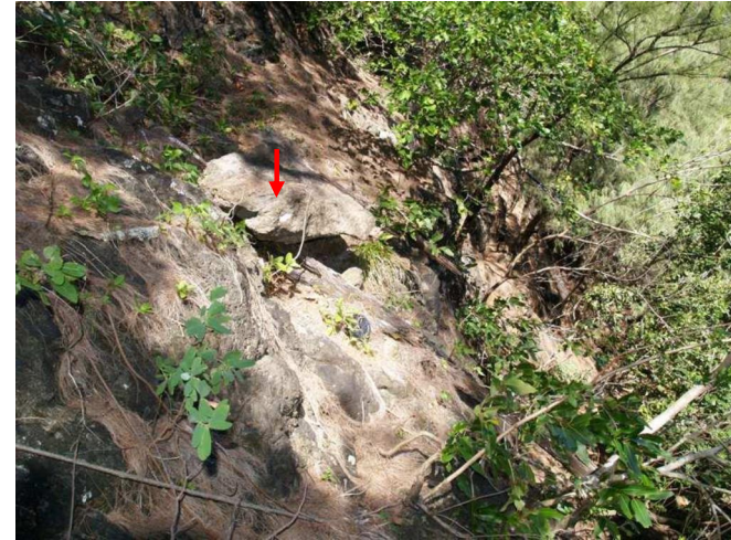
Photo 2-26. An overhanging loose rock (pointed by the arrow) sitting on top of a ledge At B26.
