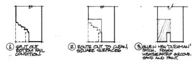
REPAIRING SPLIT-OUT BOTTOM RAIL OF SASH
