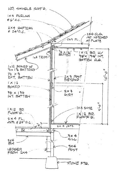
Architectural section through a board and batten wall.
