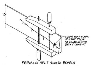
Larger cracks may require the removal of the board for repair. Carefully remove the split board without further damage. Clean surfaces of split and allow wood to dry thoroughly. Inject epoxy exterior glue into split and clamp tight. When glue has set, remove clamps, sand, and reinstall.
