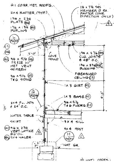
Architectural section through vertical tongue & groove board wall.
