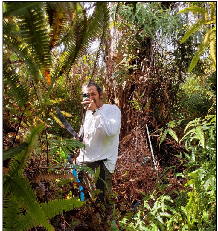
Figure 5: Forestry technician Kairos Pacheco using a relaskop to determine plot basal area.
