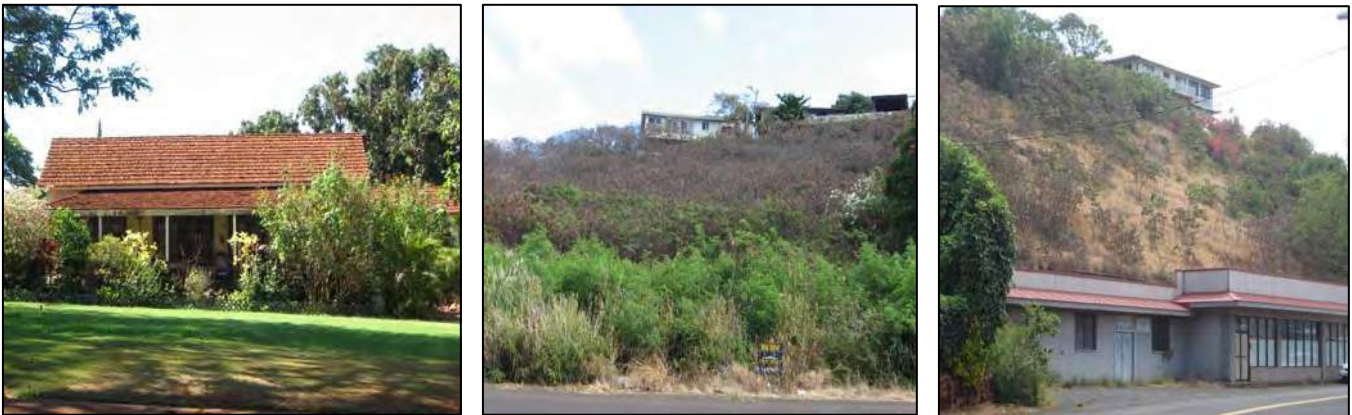
Above left: plantation home in Makaweli. Note the wood shake roof and vegetation within 10 feet of the home. Above center and right: View of houses above Hanapepe town. Note the dense dried vegetation on the hillside.
