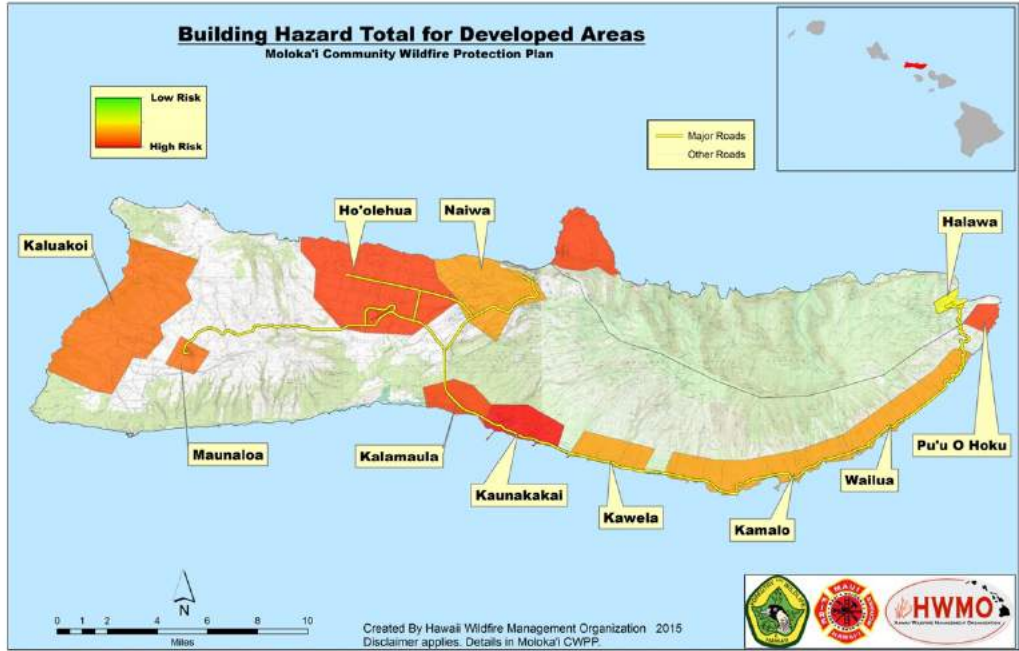
Map 20. Building Hazard Total for Developed Areas of Moloka'i CWPP planning area. Reflects hazard assessment findings related to the following categories: Siding/Soffits; Roofing Assembly; Structural Ignitability; Under Skirting Around Decks, Lanais, Post & Pier Structures; and Utilities Placement for Gas & Electric.
