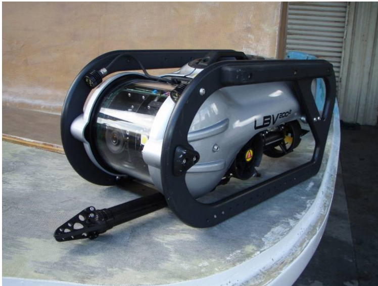
A remotely operated vehicle for carrying out hull inspections where safety or security issues affect a diver's ability to do inspections.
