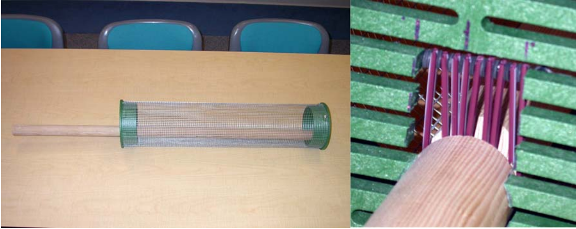
FIGURE 8. Prototype pheromone-based trap for the brown treesnake ( Boiga irregularis ). The female sex pheromone is applied to the wooden pole leading into the trap. In the field, the pole will be connected to a much longer pheromonally-inoculated guideline (not shown). The second panel shows a detail of the wooden pole leading into the trap door. Plastic bars hanging in the trap doorway swing in, allowing a snake to enter trap, but do not swing out.
