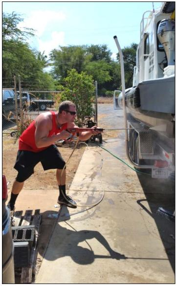
Figure 23. Pressure washing hull of NOAA vessel
