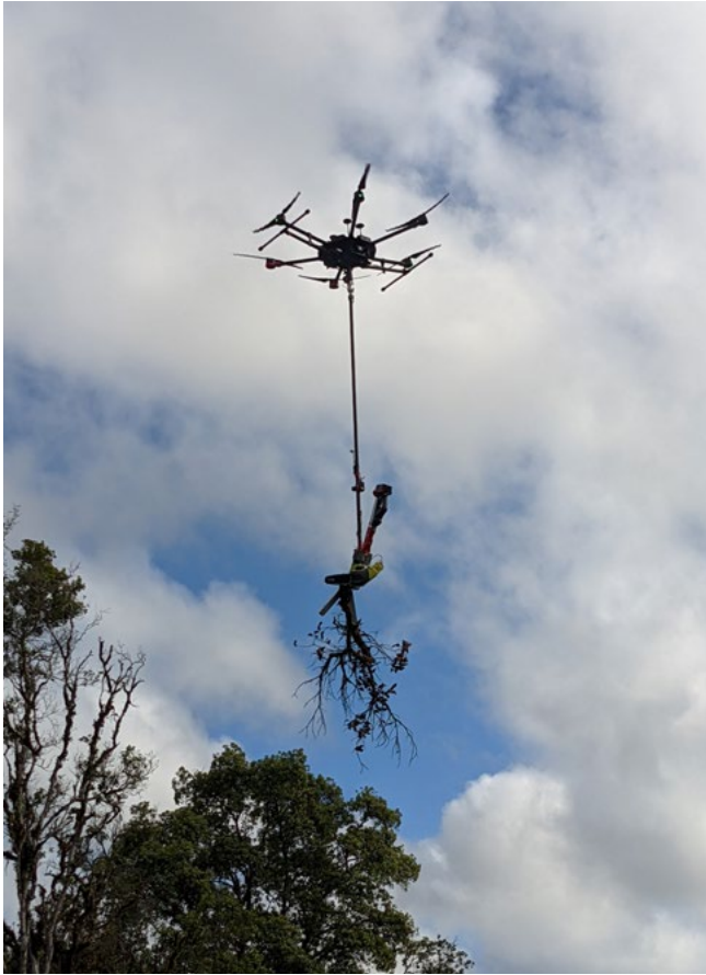
The UH SDAV Lab developed a method for cutting and sampling branches of suspected ROD-infected trees using a drone.
