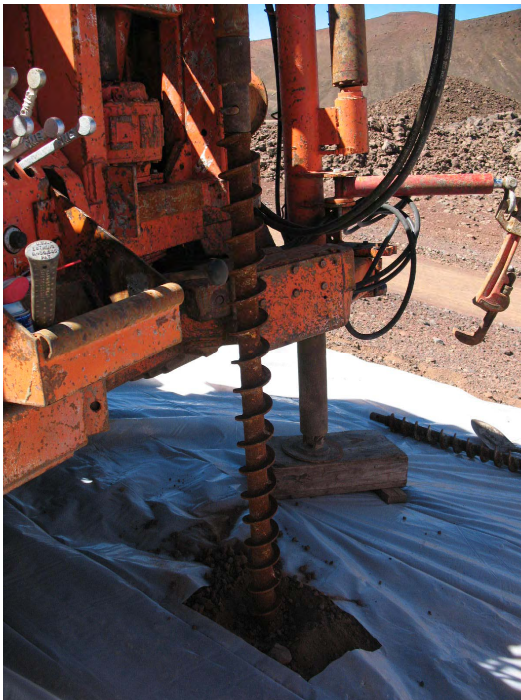
Figure 10. Auger being used at B-9.
