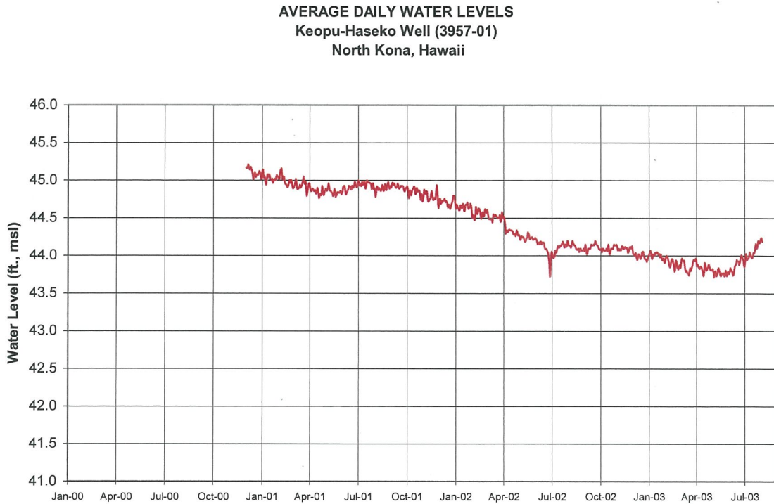
Figure 28. Average daily water levels in Keopu-Haseko well (from Daniel Lum, Water Resource Associates).
