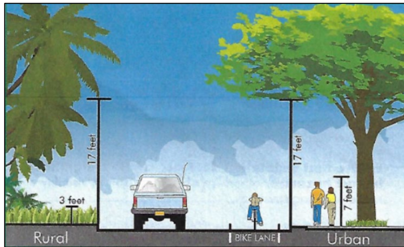
Figure 4.1 Ideal Vertical Clearance within the LMZ
