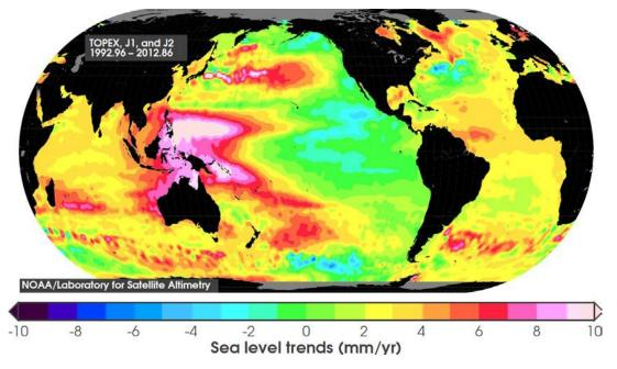
Figure B-5. Regional rates of sea level change between 1993 and present from overlapping satellite altimeter missions. (From NOAA 2010b.)
