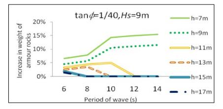
Figure C-7. Increase in the required weight of armor stone for Scenario 2, compared with no SLR. (From Esteban et al. 2011.)
