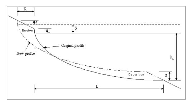
Figure D-8. Diagram of the Bruun Rule method for estimating the beach profile response to SLC.
