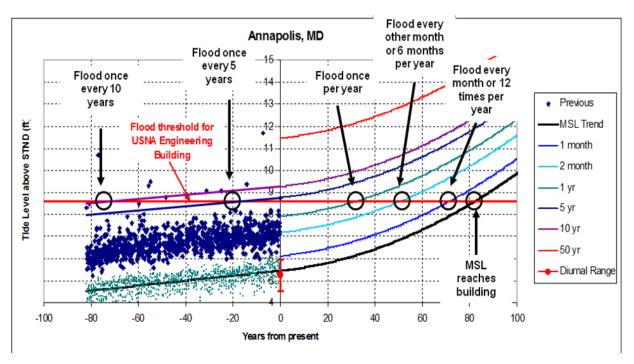
Figure C-4. Interpretation of projected SLR results and average frequency of flooding at the U.S. Naval Academy Engineering Building. (From Kriebel 2012.)
