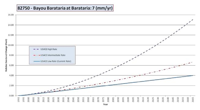
Figure E-8. Relative sea level rise curves for the nearest long-term tide gauge.
