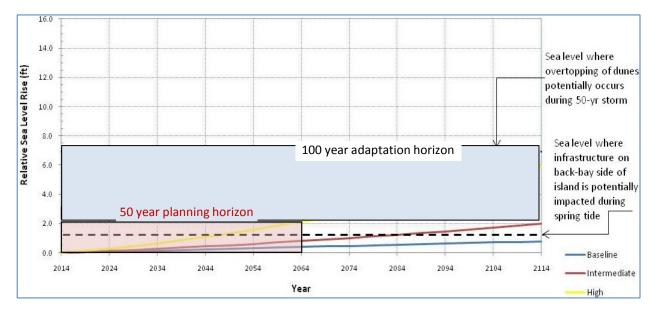
Figure 11. Topographical illustration of the project area's sensitivity to future SLC magnitudes and rates.
