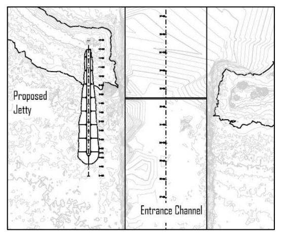
Figure C-13. Proposed jetty alignment relative to the Barber Point Harbor entrance channel. (From USACE 2012.)
