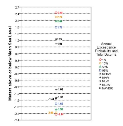
Figure B-17. Stick diagram of exceedance probability levels for Astoria, OR. (http://tidesandcurrents.noaa.gov/est/stickdiagram.shtml?stnid=9439040.)
