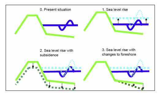
Figure E-1. Potential load cases on FDR elements under sea level rise. Relative sea level change can alter forcings on FDR infrastructure in various ways, depending on the interactions of subsidence and eustatic changes.
