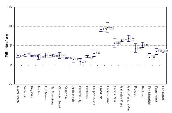
Figure B-10. Magnitude and confidence limits of trends for Florida Keys and Gulf of Mexico coast NOS tide gauges. (From Zervas 2009.)
