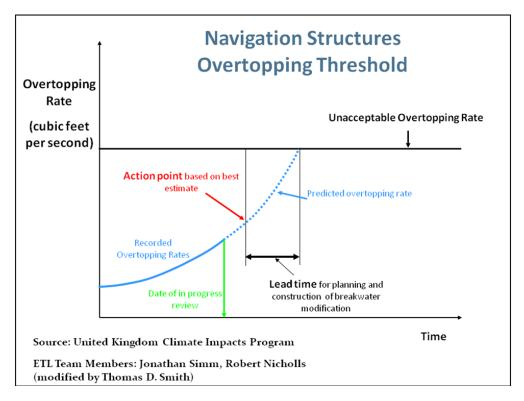
Figure C-3. Tipping point diagram for navigation structure overtopping threshold under a sea level rise scenario.
