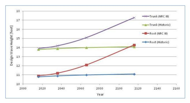
Figure C-15. Depth-limited breaking wave heights (with SLC).
