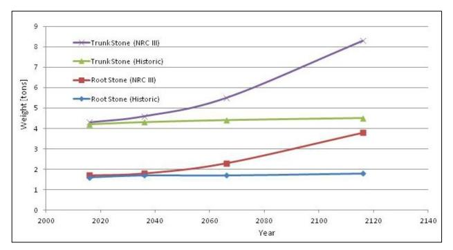
Figure C-16. Increase in Core Loc weight for the historic and USACE high curves.
