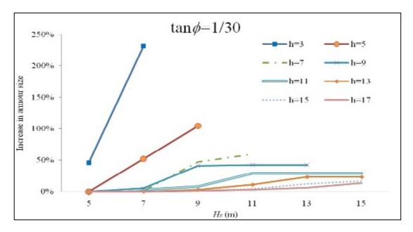
Figure C-9. Increase in armor stone size for Scenario 4 for a variety of  $H_s$  values. (From Esteban et al. 2011.)
