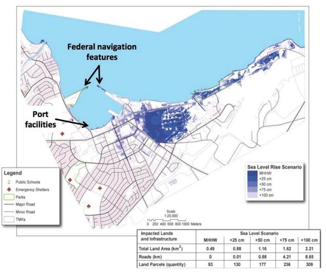
Figure C-1. Example layout of a navigation project with impacted features and areas noted. (From Cooper et al. 2012.)
