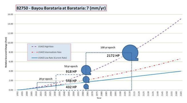
Figure E-13. Algiers SELA pump station capacity required for the three RSLR rates.
