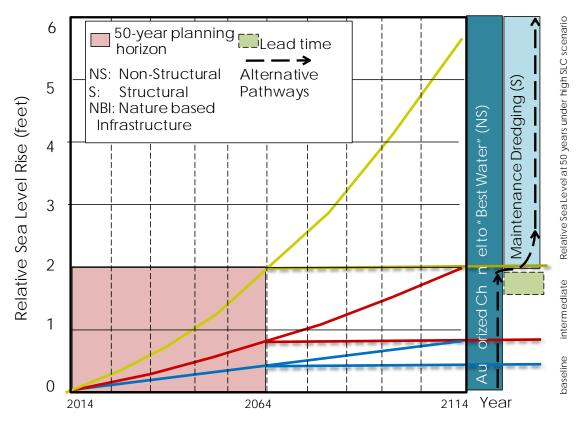
Figure C-11. Transition of a project feature over the life cycle from "best water" to maintenance dredging for the three USACE SLC planning curves (blue is low, red is intermediate, and yellow is high-rate curve).
