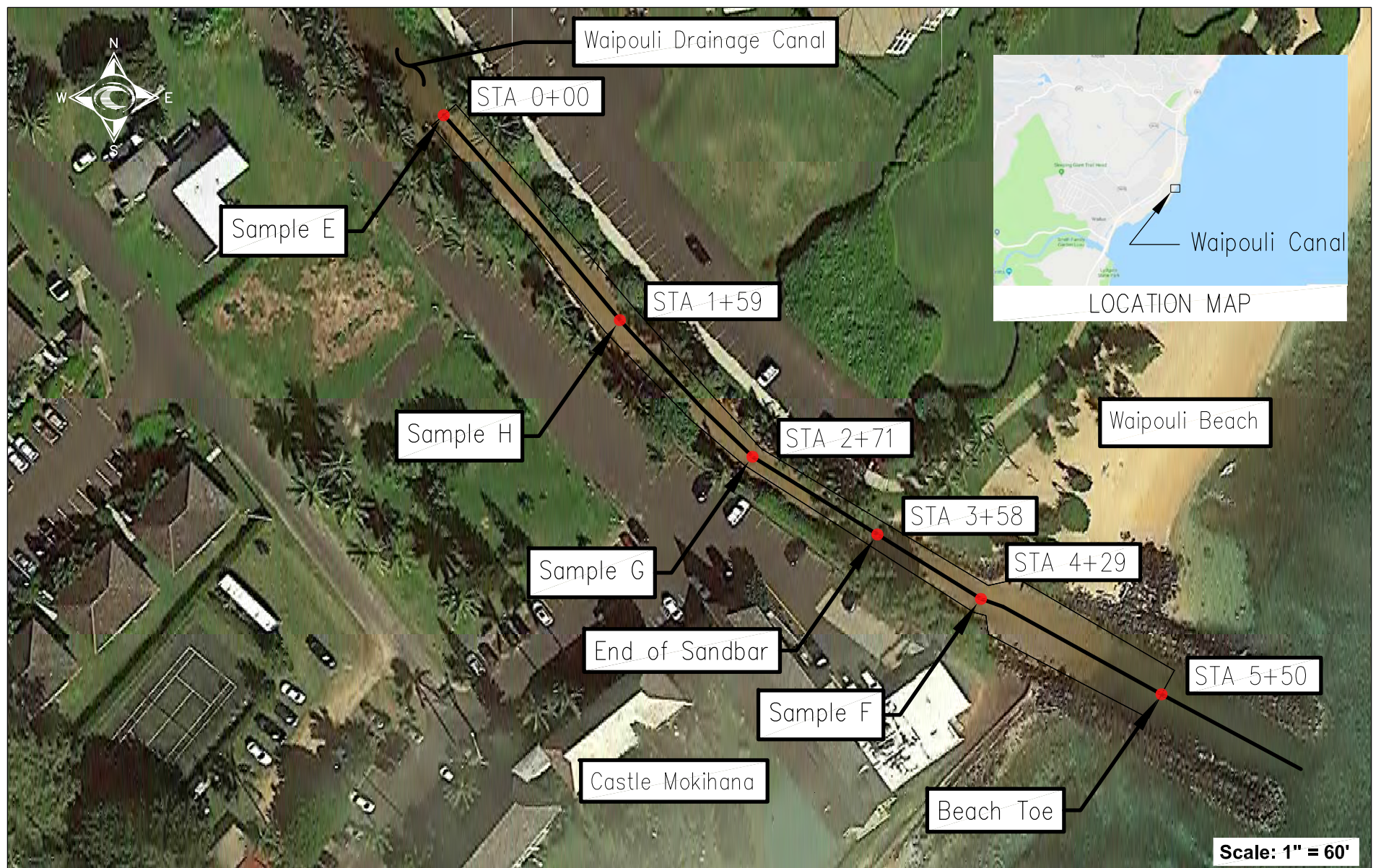
Figure 1: Waipouli Drainage Canal Sediment Sampling Plan View
