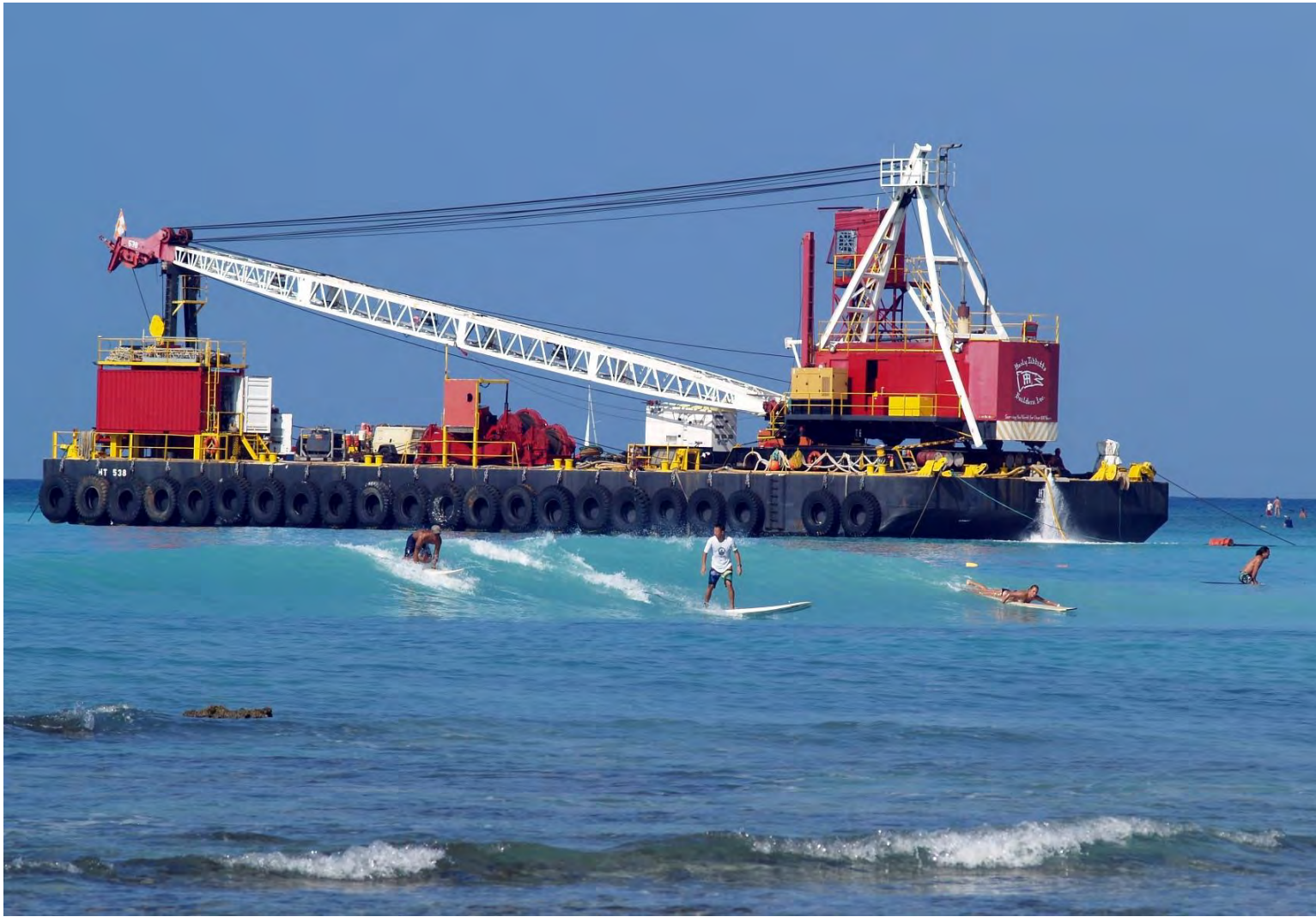
Figure 1-20. Hydraulic sand recovery system used in the 2012 Waikīkī Beach Nourishment Project
