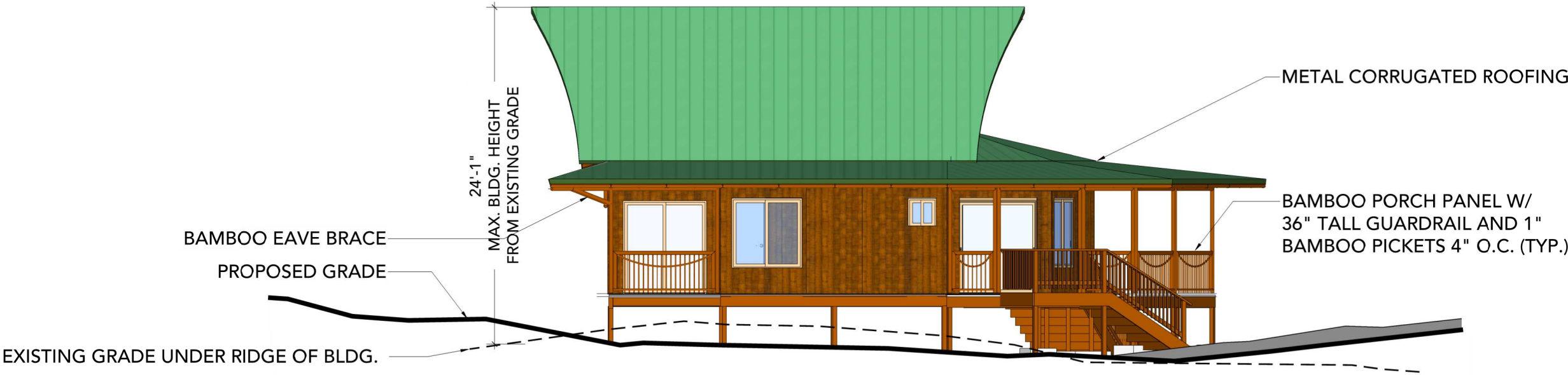
2 EAST ELEVATION SCALE: 1/8"=1'-0"
