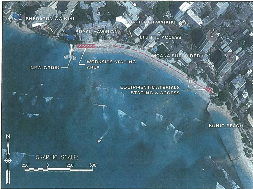
Construction access and staging areas
