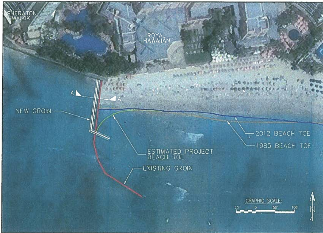
Concrete wall groin plan view
