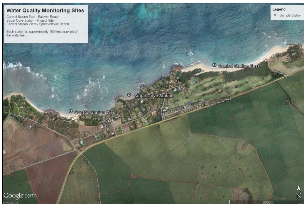
Figure 3-1. Water quality monitoring stations for turbidity sample collection
