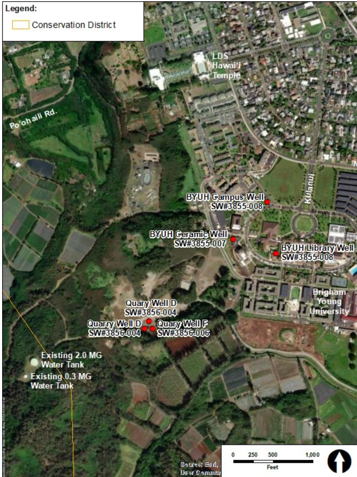
Figure 1-3: Location of Existing LWC Wells and Tanks
