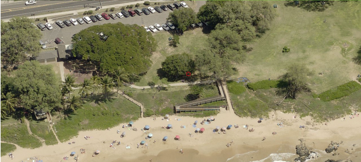
FIGURE 30. (Left) Dune ramp constructed to provide shoreline access and protect the restored dunes at Kamaole Beach Park I in Kihei, Maui. (Photo: Wes Crile, Hawai’i Sea Grant) (Bottom) Dune Walkovers at Kamaole Beach Park III in Kihei, Maui. (Photo: Eagleview Connect Explorer/County of Maui)
