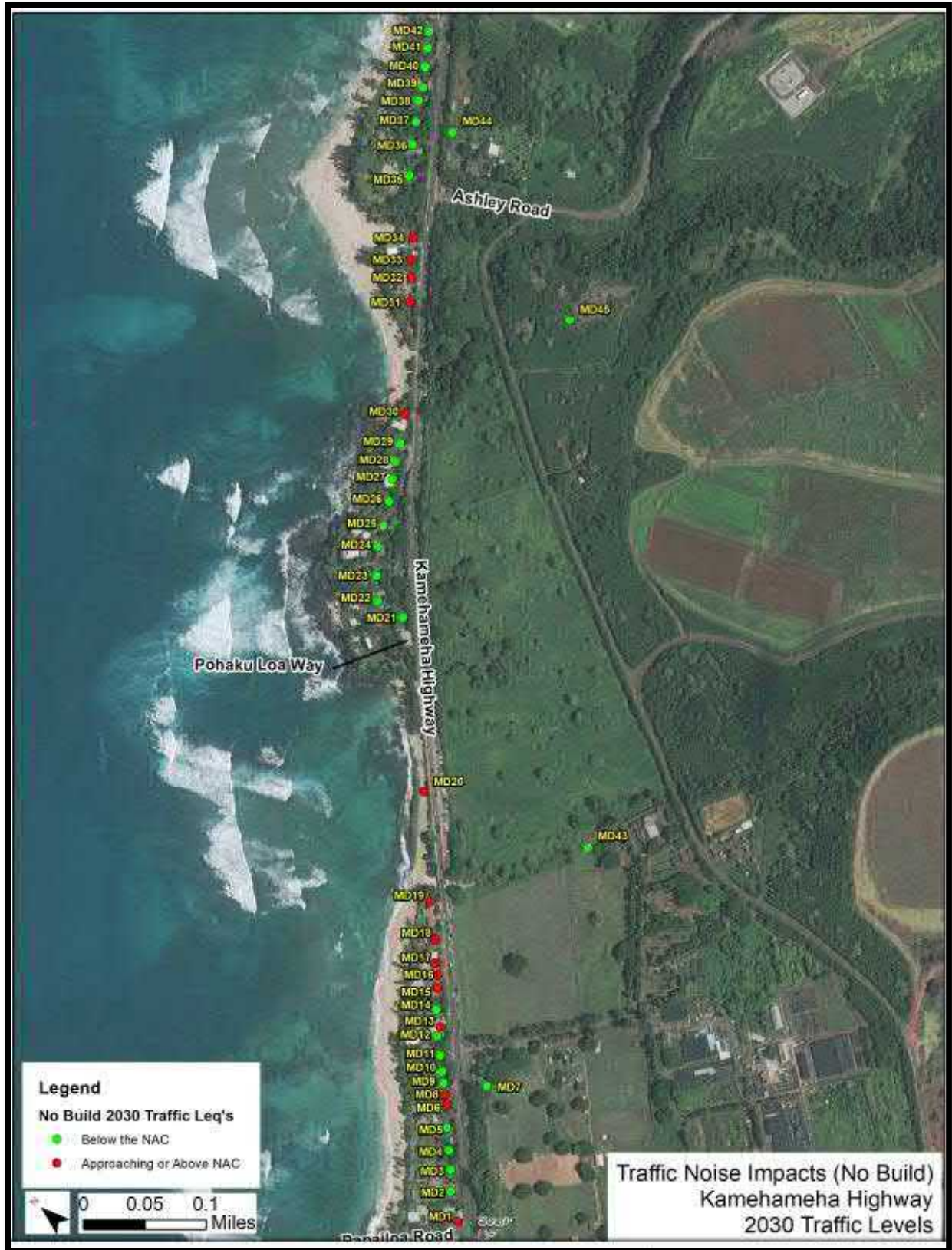
Figure 3-14. No Build Alternative Traffic Noise Impacts
