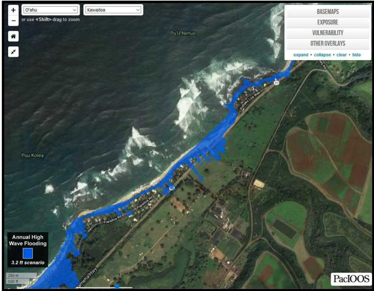
Figure 3-2. Annual High Wave Flooding at Laniakea Beach under a 3.2-foot Sea Level Rise Scenario
