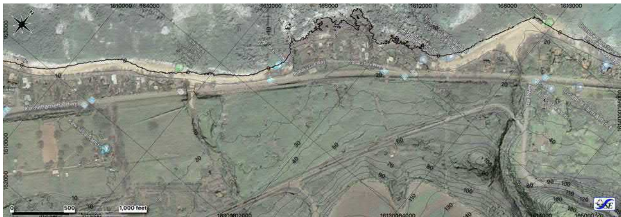
Figure 2-2. Project site with topographic contours labeled at 10 ft interval, with MSL in bold
