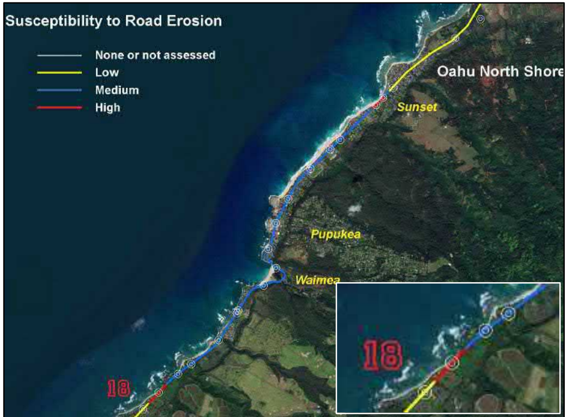
Figure 4-28. Road erosion susceptibility; inset is the project area
