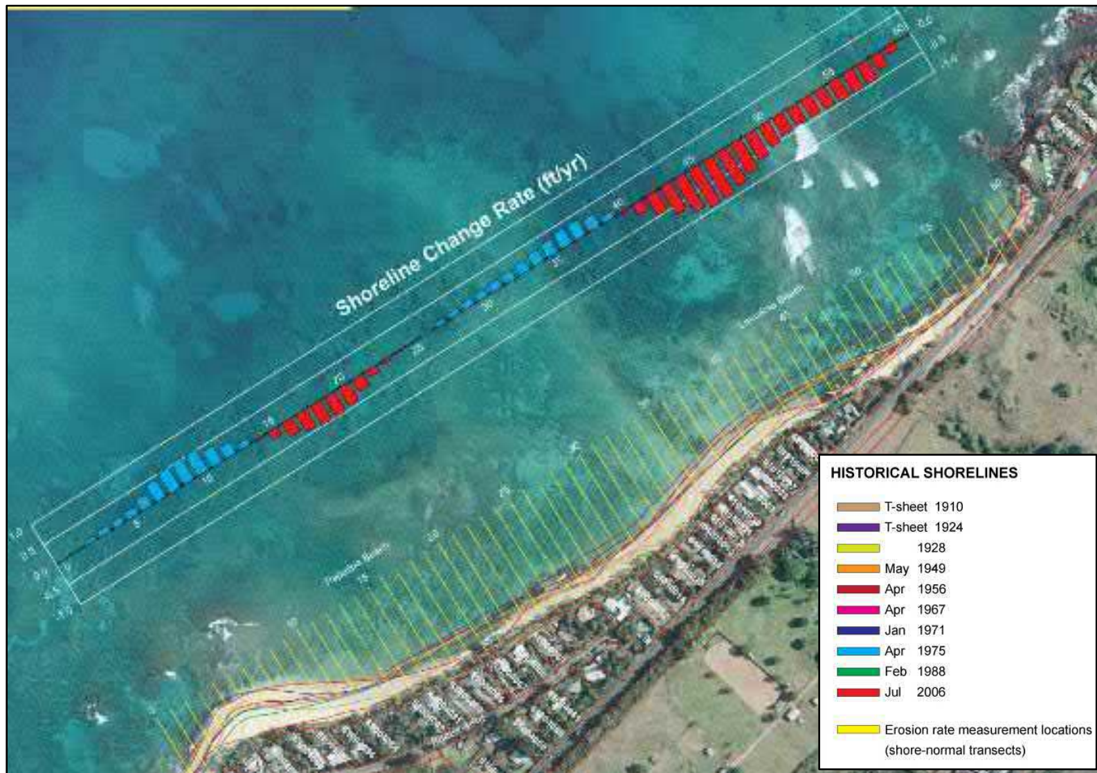
Figure 2-8. Historical aerial photograph analysis by UHCGG
