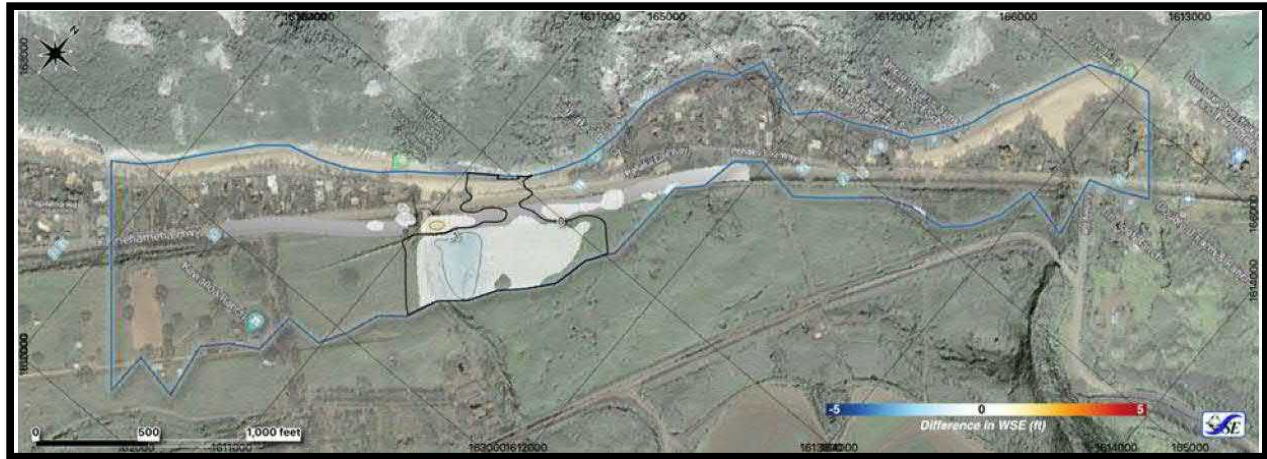
Figure 3-5. Illustration of the Difference Between the Existing Tsunami Wave Surface Elevation and Modeled Change in Wave Surface Elevation Caused by the Proposed Project (Wave Surface Elevation Contours in Feet)
