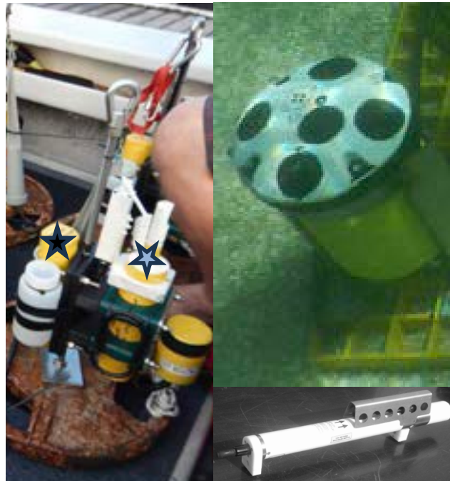
Figure B-4. Instrument Deployment #2/#3: One Nortek Signature 1000 (right); One RBR Virtuoso Dwave Logger (left; black star); One Seabird MicroCAT (bottom right); One RBR Tu (middle-bottom; blue star) Deployed Together on a Ballasted Frame with a Vertical Bar for Securing the Sensors
