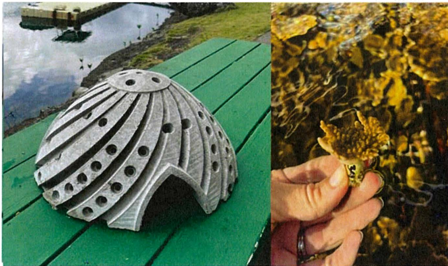
CGM (left) with pre-drilled holes to fit aragonite plugs that hold juvenile corals (right)
