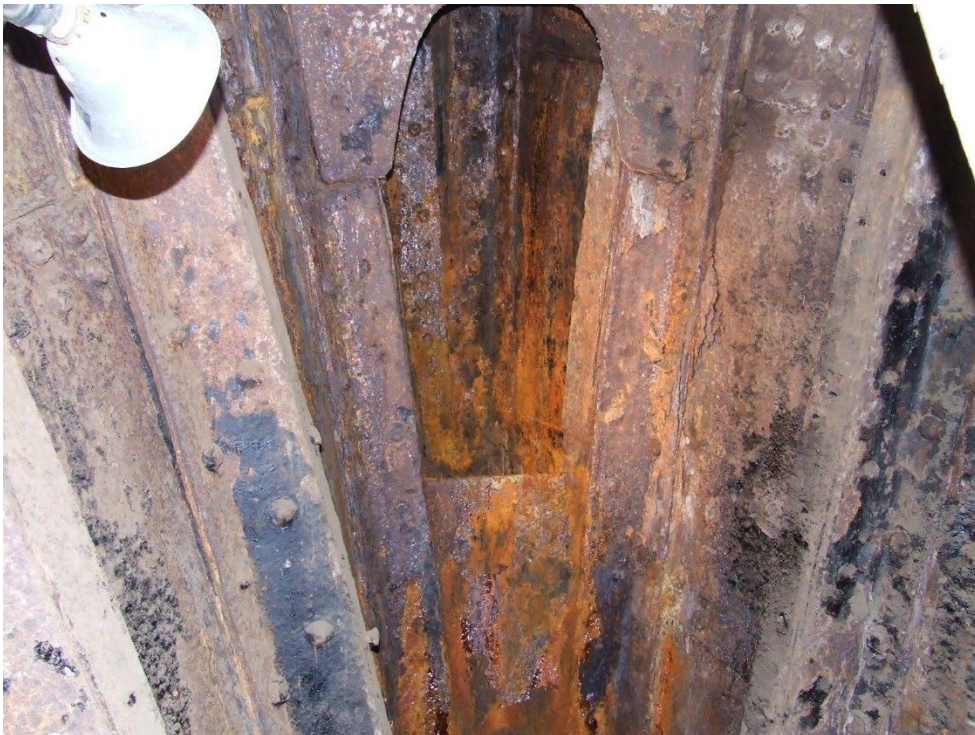
Stern casting, inboard face showing much wastage.
