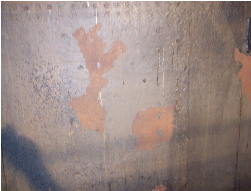
New paint system failure on bulkhead.
