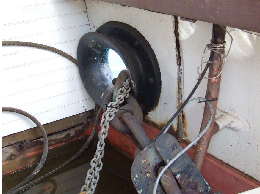
Wasted side shell plating in danger of giving away under strain from anchor rode; port side aft maindeck.
