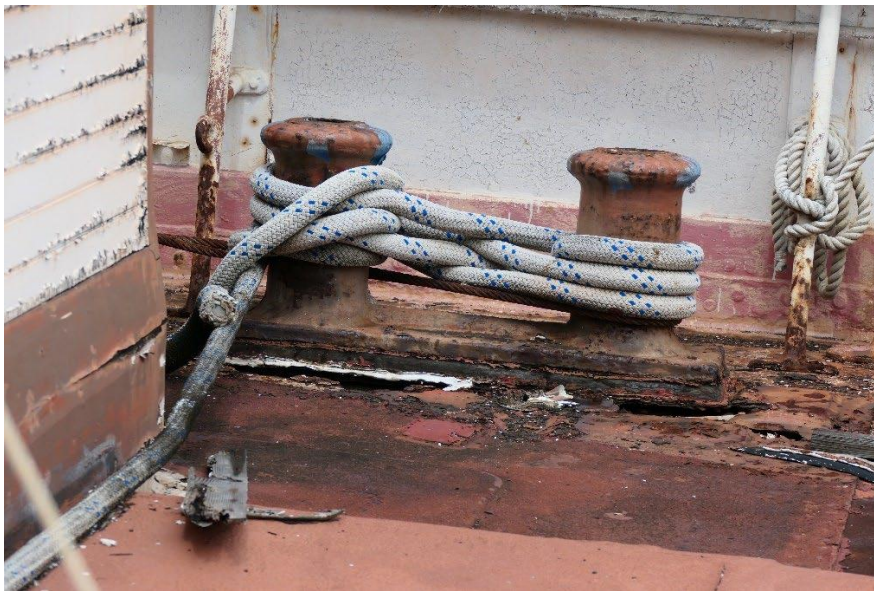
Wasted double bitts, fir foundation and deck badly corroded and rotted. Unsafe, yet still securing vessel under load.
