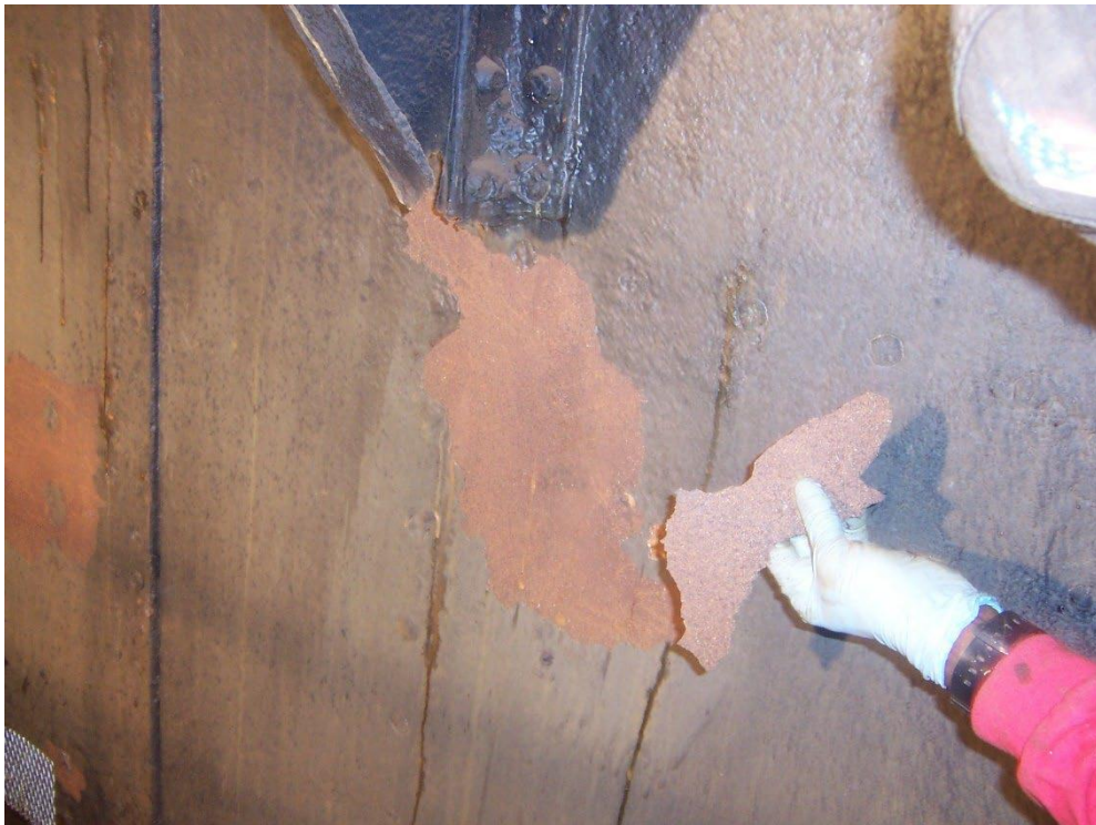
New paint system failure on bulkhead.
