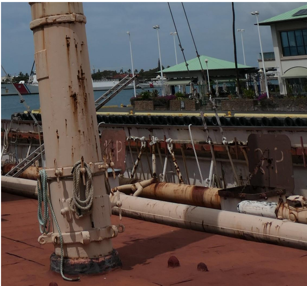
Figure 5: Chain-plates on the port side with minimal rigging for the mizzen-mast (Joseph Lombardi).
