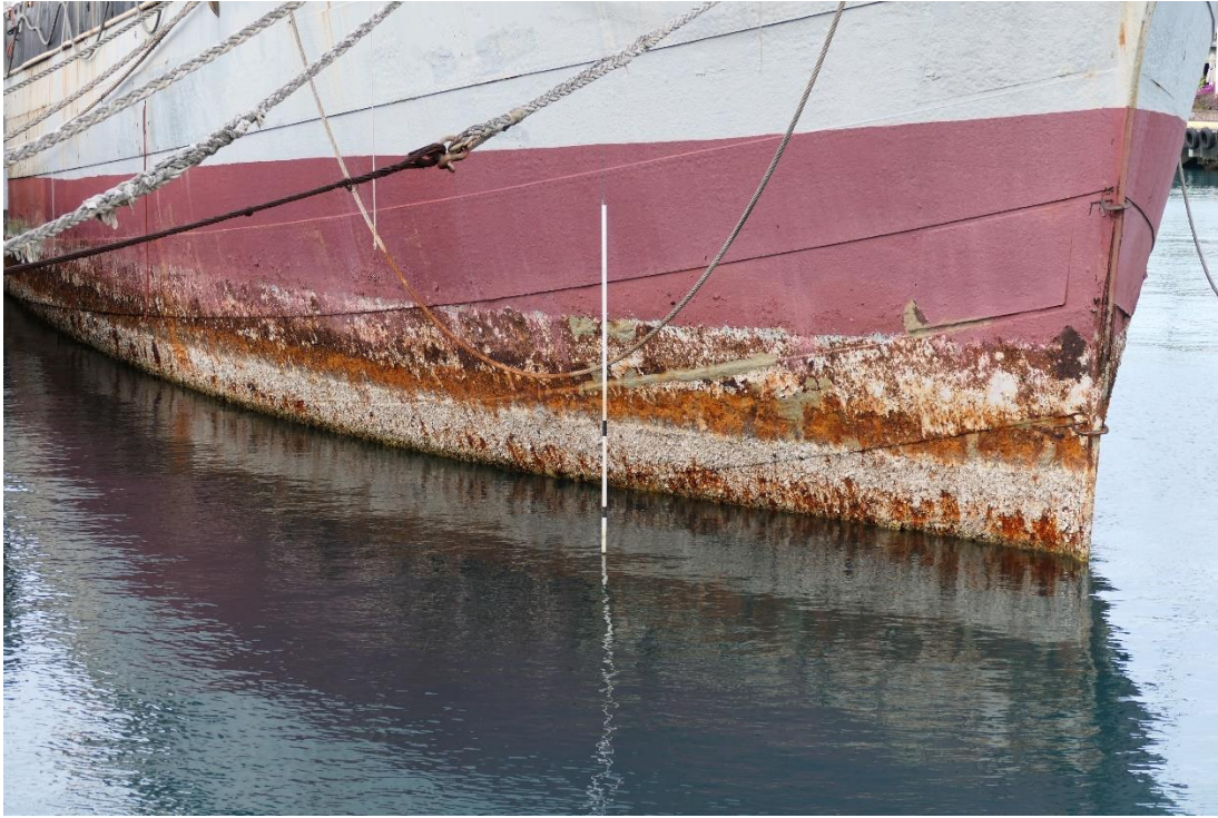
Figure 7: Condition of the lower hull, March 2023 (Joseph Lombardi).
