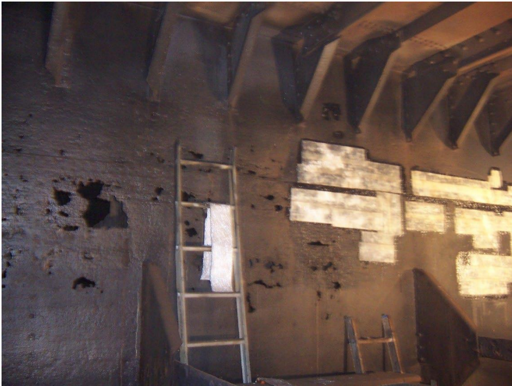
Wasted transverse bulkhead, indicative of conditions found throughout tank system. Bulkheads are Swiss cheese.
