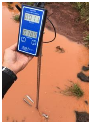
Taking flow measurements in Keokea Gulch mauka of Piilani Highway
