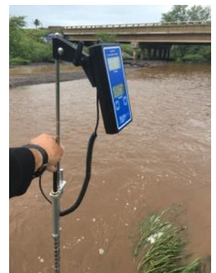
Taking flow measurements in Kulanihakoi Gulch just north of South Kihei Road.
