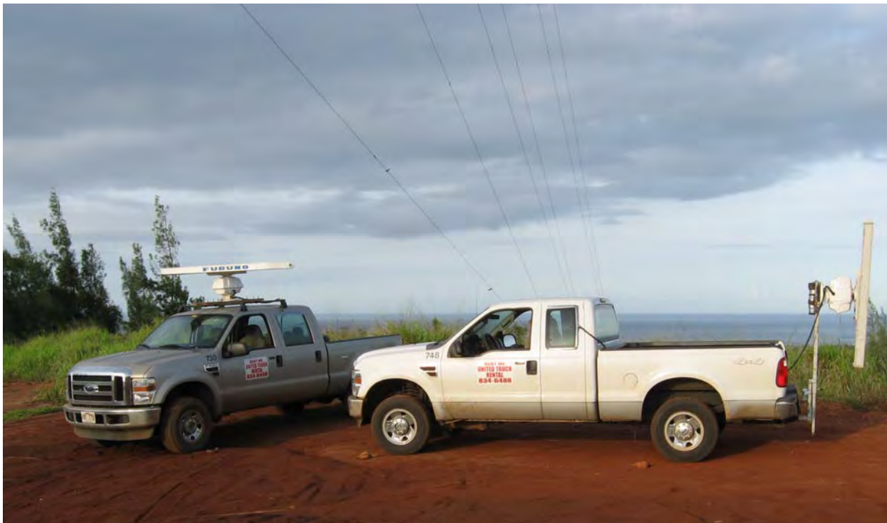
Figure 3. The surveillance and vertical radars used for studies of Newell’s Shearwater at the proposed Na Pua Makani Wind Energy Project, Oahu Island, Hawaii, fall 2012, and spring and summer 2013.
