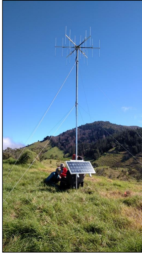
Figure 6. SigmaEight Orion automated radio receiving tower set up at site T1.
