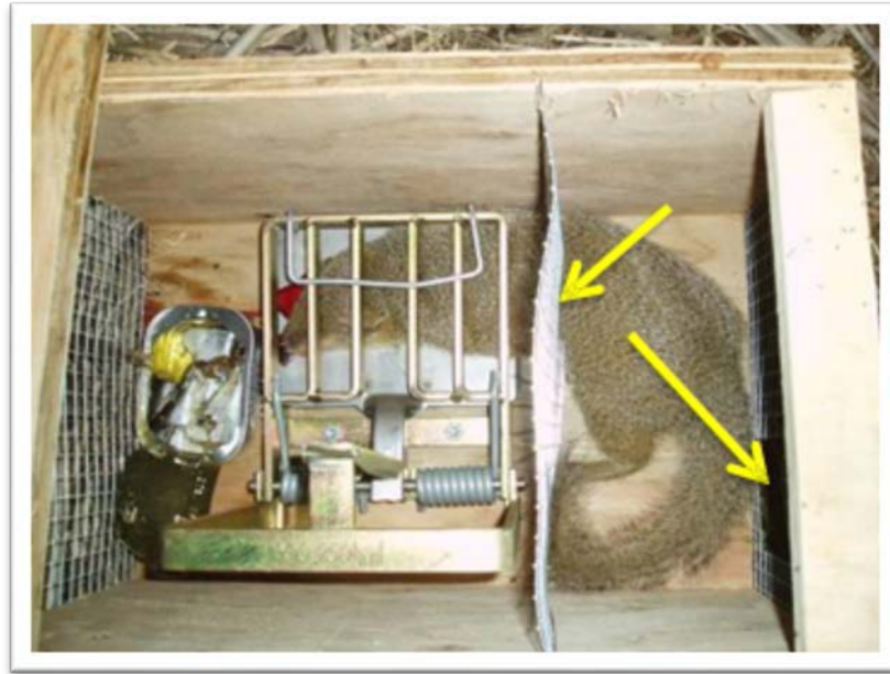
Figure 5. DOC-250 trap encased in a "bird-safe" box with arrows pointing to the 2 separate entrances that must be negotiated to access and trigger the trap mechanism itself.
