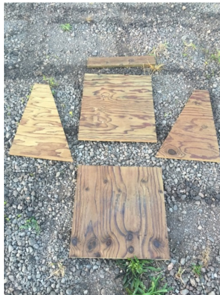
Figure 5. An insulation box prior to assembly
