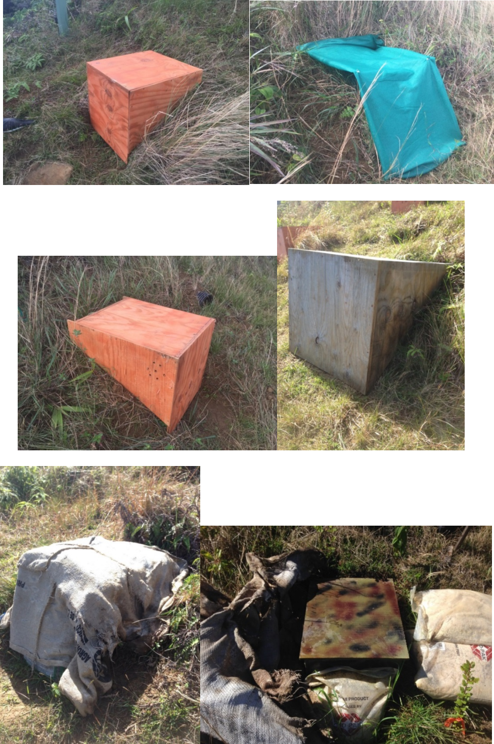
Figure 2. Each of the experimental insulation designs tested. Left top: Small unvented. Right top: Shade cloth. Mid left: Small vented. Mid right: Large insulated. Bottom: sand bag and burlap burrow covered left and exposed right.
