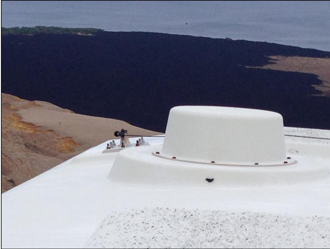
Figure 2. Bat detector microphone mounted on nacelle.
