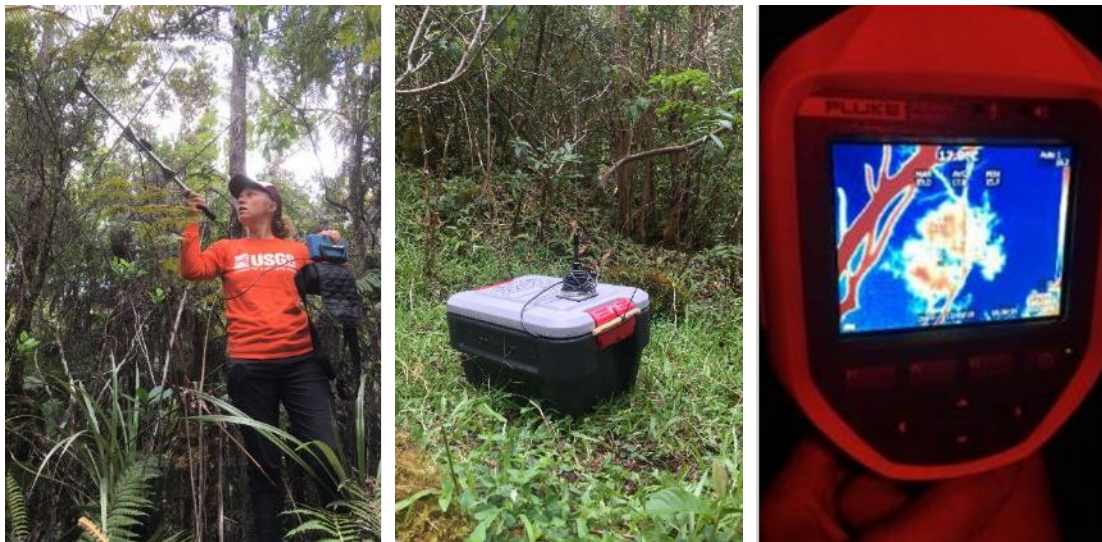
Figure 3. Radio telemetry effort to located day roost tree (left). Automated receiver station used to measure roost fidelity (middle). Thermal imager used for searches for roosting bats (right).
