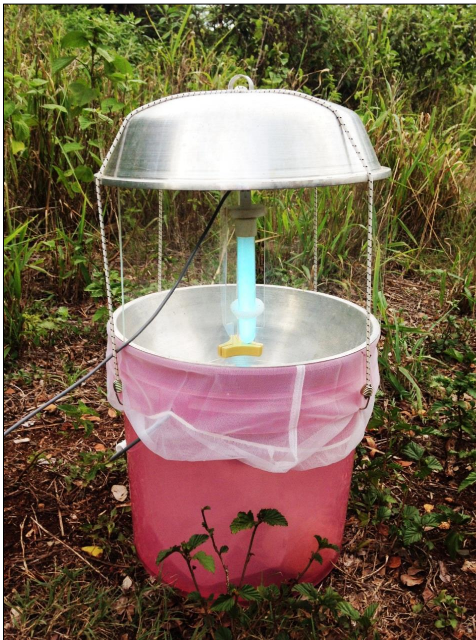
Figure 6. Light9, a universal black light trap deployed in the uplands of the eastern region of 'Uko'a Wetland during the 2014/2015 surveys.
