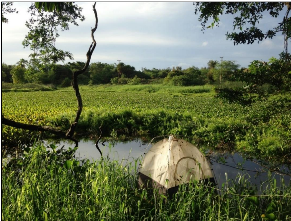
Figure 8. WaterKayak, an Aquatic Emergence Trap, that floated on open water in the northeastern corner of 'Uko'a Wetland during the 2014/2015 surveys.
