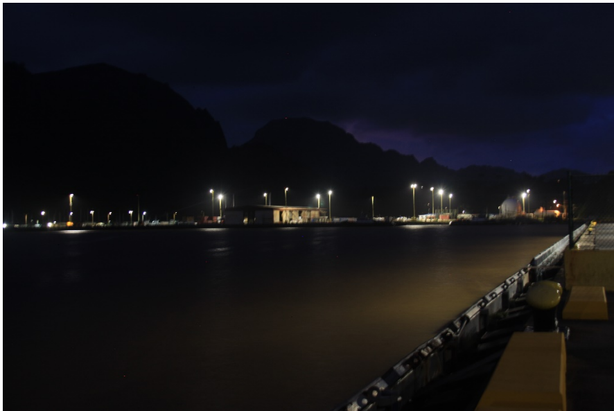
Photo 6. Lighting conditions at Pier 3 (Young Brothers yard) during non-operational security conditions when all high mast lights are reduced to 15% illumination level.
