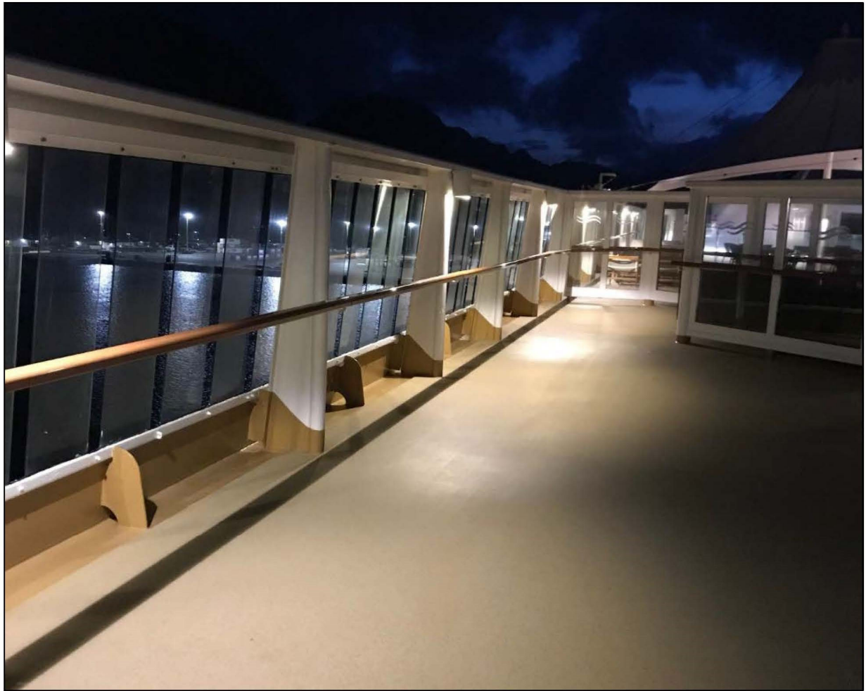
Figure 1. Deck 13, wall-mounted light fixtures configured so that light is emitted downward only (page 13).
