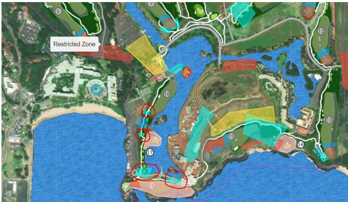
Carts automatically reduce speed when entering red areas. If cart speed is over 7 mph, cart will shut down automatically.
