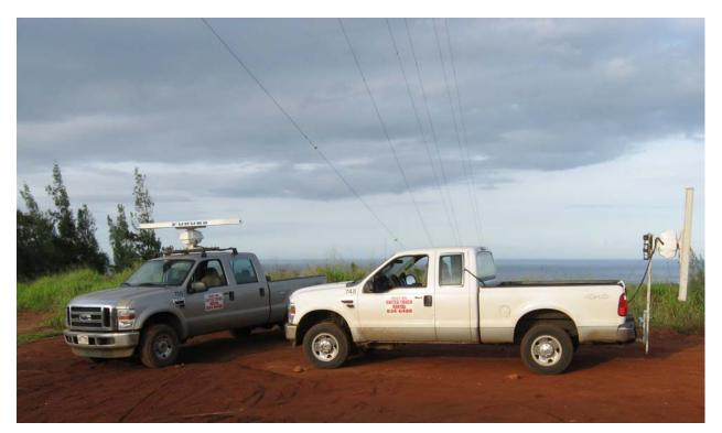
Figure 3. The surveillance and vertical radars used for studies of Newell's Shearwater at the proposed Na Pua Makani Wind Energy Project, Oahu Island, Hawaii, fall 2012, and spring and summer 2013.
