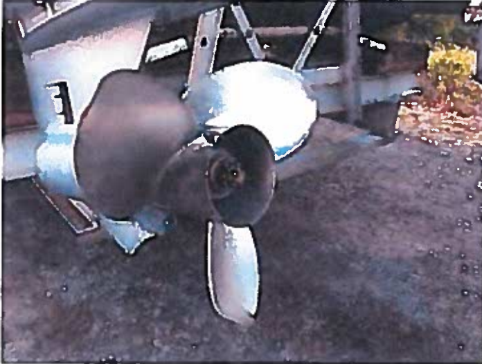
5 Depicts damage to port side motor fin
