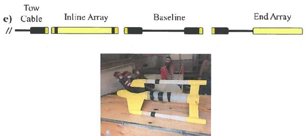
The tetrahedral array is approximately 1m long and 0.5m diameter, and consist of 4 hydrophones and an accelerometer. The hydrophones are arranged so that at least 2 are outside of the linear plane, therefore allowing for 3-D localization of a sound source. The accelerometer provides orientation information for the tetrahedral components so that the source location is accurate with respect to the horizon.
