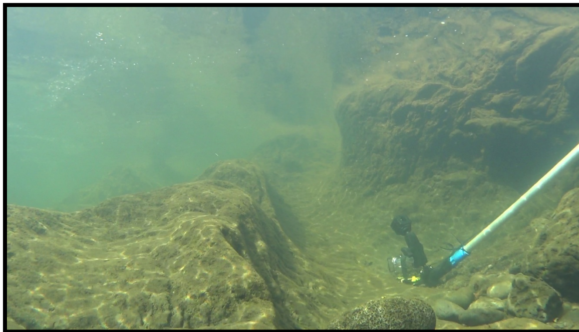
Figure 13: Underwater geo-referenced video camera with external video light used for the HDFS observations.
