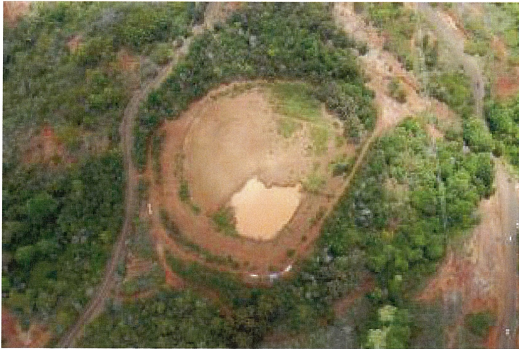
Kitano Reservoir (KA-0004) Erosion Gullies and Trees on the Upstream Slope
