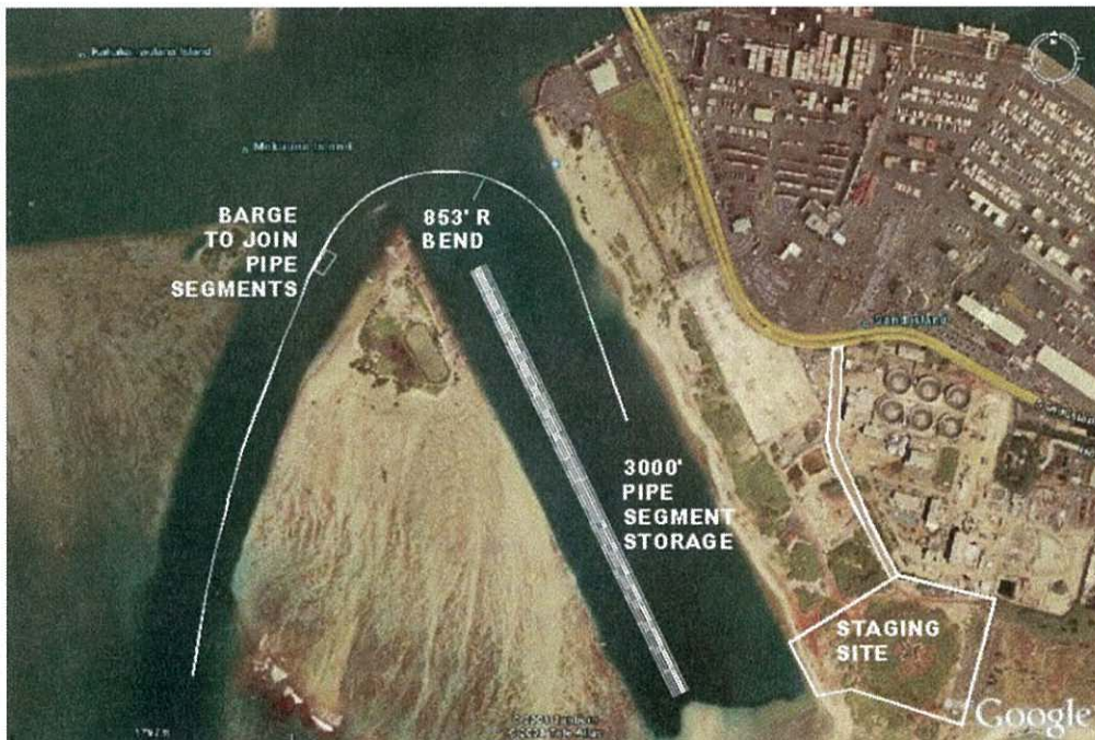
Figure 7. Plan for Connecting Pipe Segments and Towing From Ke'ehi Lagoon Source: Makai Ocean Engineering, Inc. (FEIS, HSWAC) (Cardno TEC, Inc., 2014)
