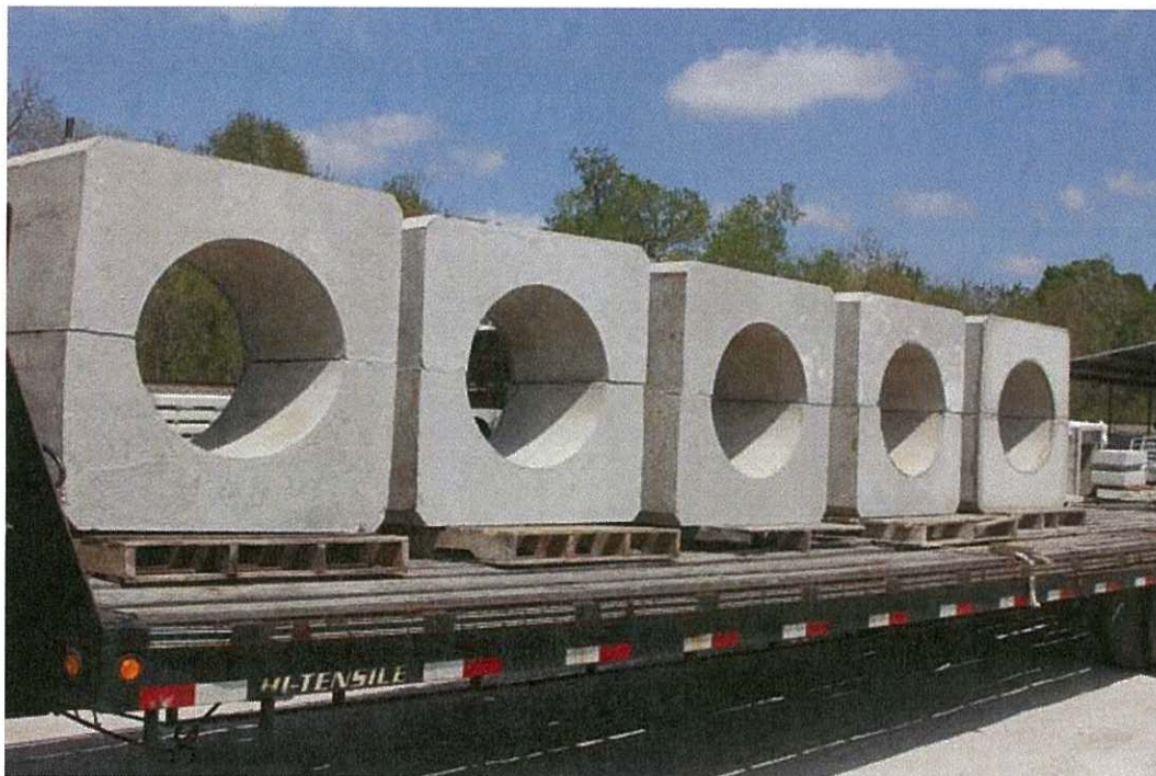
Photo 5. Example of smaller collars for deeper water sections; similar to proposed “Type C” collars (3.6 square feet area each). Source: Makai Ocean Engineering, Inc. ( https://www.makai.com/ )
