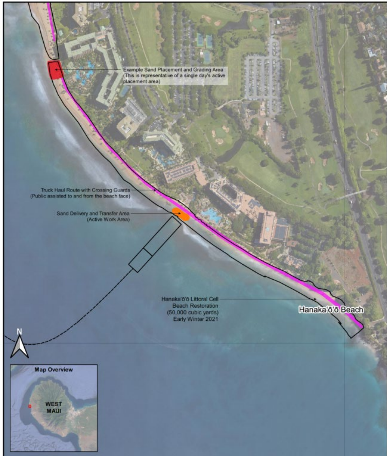
Figure 5. Hanaka'ō'ō Beach Restoration sand transfer, truck haul route, and typical daily work area.
