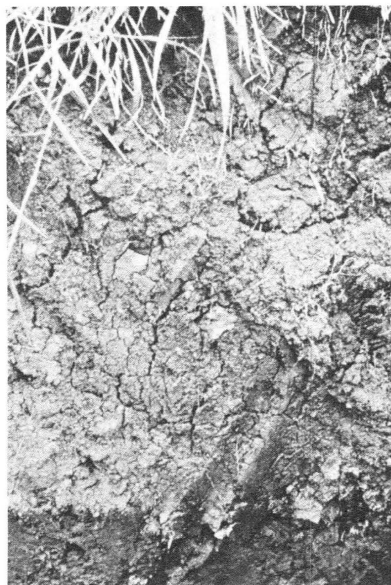
Cracks in Vertisols are open for 90 days or more each year. Some cracks extend to a depth of 40 inches (1 meter).
