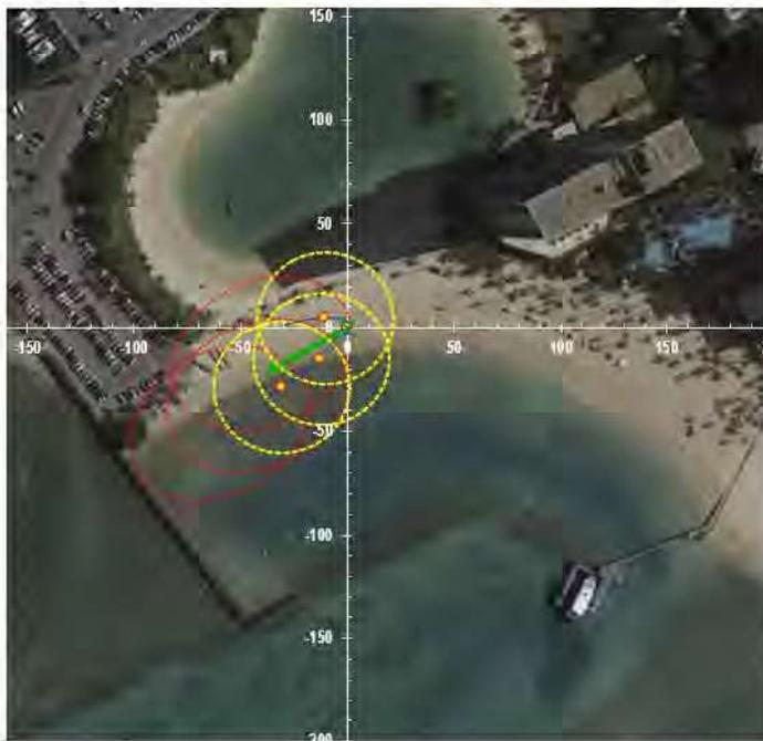
**Figure 1.** Ballistic Trajectory of the weekly display. The green x indicates the launch site, and the green arrow indicates wind direction. The blue lines indicate aerial shell trajectories, the orange dots the expected break point and yellow dotted lines the burst radius. The dotted red lines indicate the maximum expected debris fallout range.
