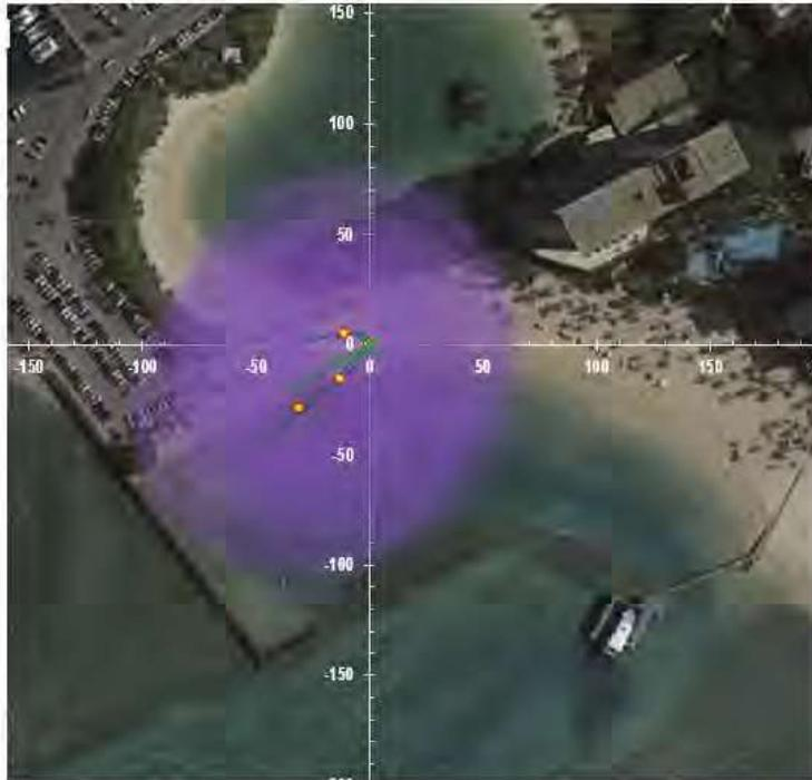
**Figure 3.** Predicted area of sound intensity of 120dB when using salute shells
