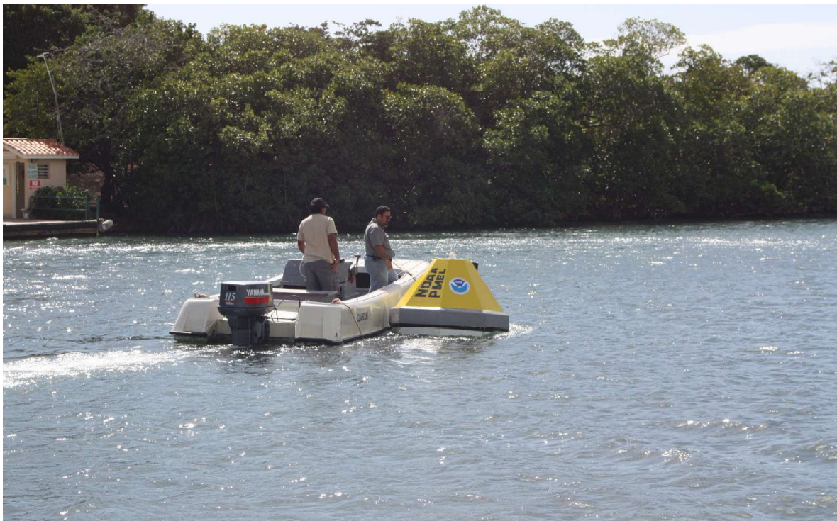
Figure #13: Towing the MApCO2 O-A buoy out to the deployment site
