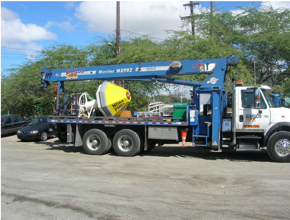
Figure #11: A typical flatbed boom truck, available for rent in many parts of the world, is a great tool for getting the buoy and anchors into the water
